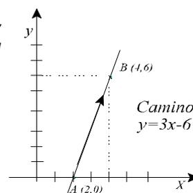
$$\begin{aligned} W_{A \rightarrow B} &= \int_{(2,0)}^{(4,6)} (-2x\hat{i} + 10\hat{j}) \cdot (dx\hat{i} + dy\hat{j}) = -\int_2^4 2x dx + \int_0^6 10 dy = -\left[ x^2 \right]_2^4 + \left[ 10y \right]_0^6 = \\ &= -12J + 60J = \underline{\underline{48J}} \end{aligned}$$
