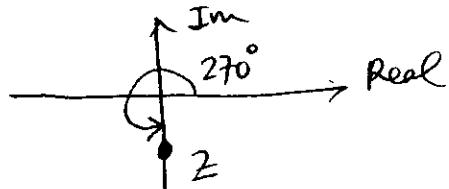
$$r = |b| \\ \alpha = 270^\circ = \frac{3\pi}{2} \text{ rad} \quad \left\{ \begin{array}{l} z = bi = |b| e^{270^\circ} \end{array} \right.$$
