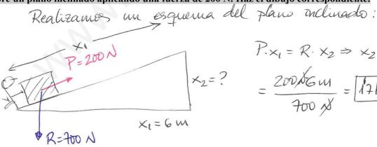
$$P. \times_{1} = R. \times_{2} \Rightarrow \times_{2} = \frac{P. \times_{1}}{R} = \frac{200 \times 6 \text{ M}}{700 \times 8} = \boxed{171 \text{ M}}$$
