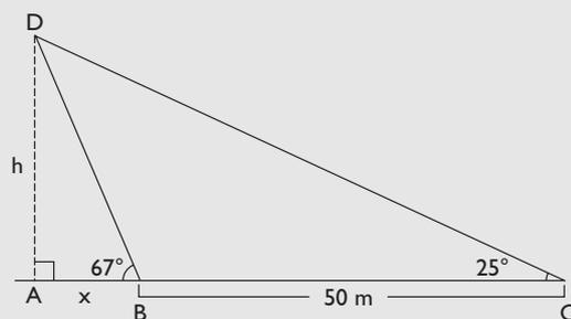
$$\left. \begin{aligned} \operatorname{tg} 67^\circ &= \frac{h}{x} \\ \operatorname{tg} 25^\circ &= \frac{h}{50 + x} \end{aligned} \right\}$$
