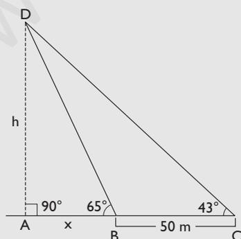
$$\left. \begin{aligned} \operatorname{tg} 65^\circ &= \frac{h}{x} \\ \operatorname{tg} 43^\circ &= \frac{h}{50+x} \end{aligned} \right\}$$
