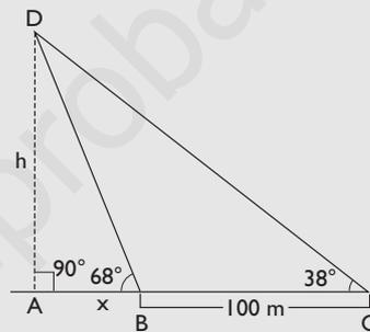
$$\left. \begin{aligned} \operatorname{tg} 68^\circ &= \frac{h}{x} \\ \operatorname{tg} 38^\circ &= \frac{h}{100 + x} \end{aligned} \right\}$$
