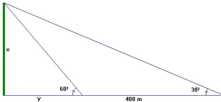
$$9. \left. \begin{array}{l} \text{tg } 30^\circ = \frac{x}{y+400} \\ \text{tg } 60^\circ = \frac{x}{y} \end{array} \right\} \rightarrow \left. \begin{array}{l} 0,58(y+400) = x \\ 1,73y = x \end{array} \right\} 0,58y + 232 = 1,73y \rightarrow 1,15y = 232$$
