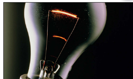
Figure 5.17 The metal filament in a light bulb glows as the current passes through it. It is also very hot. This shows that electrical energy is converted into both thermal energy and light.
