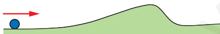
Figure 12.18 The total energy of the ball is not enough to go over the barrier so the ball will not go over the barrier.
