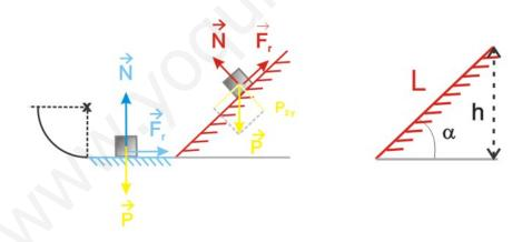
$$\begin{aligned} W_r &= -F_r L = -\mu N \frac{h}{sen\alpha} = -\mu m g \cos\alpha \frac{h}{sen\alpha} = -20.8 J \\ W_r &= -F_r d = -\mu N d = -\mu m g d = -1.2 J \\ W_{rtotal} &= W_r + W_r = -22 J \end{aligned}$$
