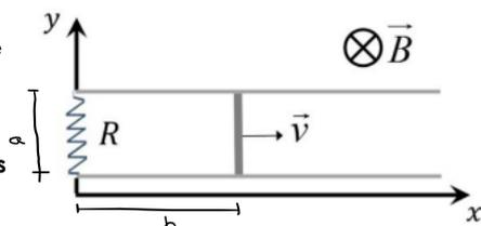
a)  $l = 20\text{cm} = 0.2\text{m} = a$     ①  $\Phi = \int \vec{B} \cdot d\vec{S} = \int B \cdot dS \cdot \cos\alpha \rightarrow \Phi = B \cdot \cos\alpha \cdot S \Rightarrow \Phi = B \cdot S \cdot \cos\alpha$
