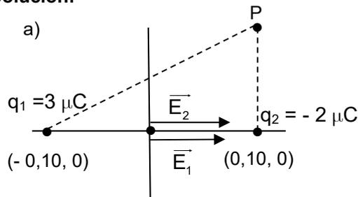
$$\vec{E}_1 = K \frac{q_1}{r_1^2} (\vec{u}_1) = 9 \cdot 10^9 \frac{\text{N m}^2}{\text{C}^2} \frac{3 \cdot 10^{-6} \cancel{\text{C}}}{0,10^2 \cancel{\text{m}^2}} \vec{i} = 2,7 \cdot 10^6 \vec{i} \left( \frac{\text{N}}{\text{C}} \right)$$
