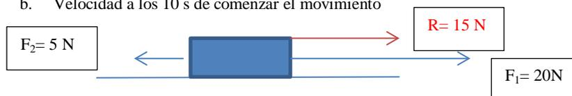
$$\sum F_i = F_1 - F_2 = 20 - 5 = 15 \text{ N} = R; \quad R = m \cdot a; \quad 15 = 2 \cdot a; \quad a = 7.5 \frac{\text{m}}{\text{s}^2}; \quad x = \frac{1}{2} \cdot a \cdot t^2; \quad x = \frac{1}{2} \cdot 7.5 \cdot 9 = 33.75 \text{ m}$$
