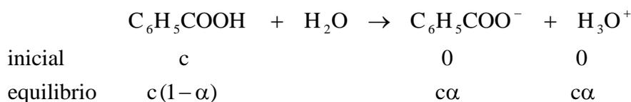
$$K_a = \frac{[C_6H_5COO^-] \cdot [H_3O^+]}{[C_6H_5COOH]} = \frac{c^2 \alpha^2}{c(1-\alpha)} = \frac{c \cdot \alpha^2}{(1-\alpha)} \approx c \cdot \alpha^2 \Rightarrow \alpha = \sqrt{\frac{K_a}{c}} = \sqrt{\frac{6'5 \cdot 10^{-5}}{0'05}} = 0'036$$
