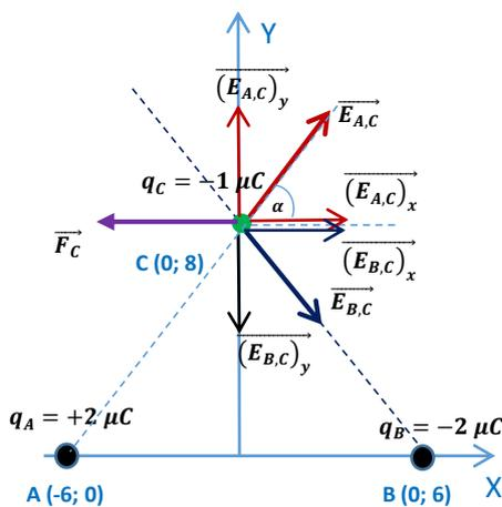
$$r_{A,C} = r_{B,C} = r = \sqrt{(6)^2 + (8)^2} = 10 \text{ m}$$
