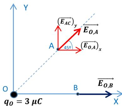
$$r_{OB} = 6 \text{ m}; \quad r_{OA} = \sqrt{4^2 + 4^2} = \sqrt{32} \text{ m}$$
