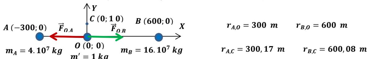
$$\vec{F}_O = \vec{F}_{O,A} + \vec{F}_{O,B} = G \cdot \frac{m_A \cdot m'}{(r_{A,O})^2} \cdot (-\vec{i}) + G \cdot \frac{m_B \cdot m'}{(r_{B,O})^2} \cdot \vec{i} = G \cdot m' \cdot \left( \frac{m_B}{(r_{B,O})^2} - \frac{m_A}{(r_{A,O})^2} \right) \cdot \vec{i}$$
