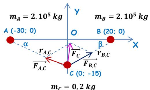
$$\vec{F}_C = G \cdot m_C \cdot \left[ \frac{m_A}{(r_{A,C})^2} \cdot (-\cos 26,56^\circ \vec{i} + \sin 26,56^\circ \vec{j}) + \frac{m_B}{(r_{B,C})^2} \cdot (\cos 36,87^\circ \vec{i} + \sin 36,87^\circ \vec{j}) \right]$$
