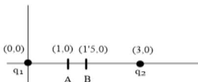
$$\vec{E}(A) = 0 = \vec{E}_{q_1}(A) + \vec{E}_{q_2}(A) \Rightarrow |\vec{E}_{q_1}(A)| = |\vec{E}_{q_2}(A)| \Rightarrow K \cdot \frac{q_1}{1^2} = K \cdot \frac{q_2}{2^2} \Rightarrow 4q_1 = q_2$$
