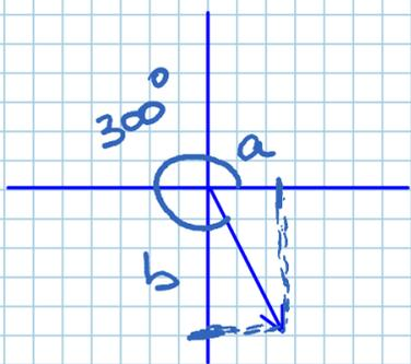
$$\begin{aligned} a &= r \cos \alpha = 3 \cos 300^\circ = 3 \cdot \frac{1}{2} = \frac{3}{2} \\ b &= i r \sin \alpha = 3 \sin 300^\circ i = 3 \cdot \left(-\frac{\sqrt{3}}{2}\right) i = -\frac{3\sqrt{3}}{2} i \\ \text{Binómica} &= \frac{3}{2} - \frac{3\sqrt{3}}{2} i & \text{trigonométrica} &= 3(\cos 300^\circ + i \sin 300^\circ) \end{aligned}$$
