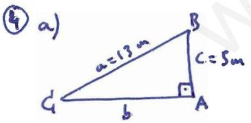
$\text{sen} C_1 = \frac{c}{a} \Rightarrow \text{sen} C_1 = \frac{5}{13} \Rightarrow C_1 = \text{arcsen} \frac{5}{13} \approx 22^\circ 37' 12'' \Rightarrow B = 90 - C_1 \approx 67^\circ 22' 48''$
