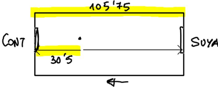
$$\begin{array}{r} 105'75 \\ 30'50 \\ \hline 075,25 \end{array} \quad \begin{array}{l} \text{la dist. será} \\ \text{de } 75'25 \text{ m} \end{array}$$
