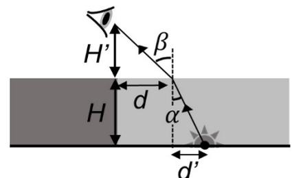
$$\begin{aligned} n \sin \beta &= n_{\text{agua}} \sin \alpha \rightarrow \sin \alpha = \frac{n}{n_{\text{agua}}} \sin \beta = \\ &= \frac{n}{n_{\text{agua}}} \frac{d}{\sqrt{H'^2 + d^2}} = \frac{1}{1,33} \frac{1,2}{\sqrt{1,6^2 + 1,2^2}} = 0,45 \rightarrow \alpha = 26,74^\circ \end{aligned}$$
